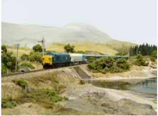
The layout is fully signalled and utilises etched brass semaphore signals which are operated using Fulgurex point motors. The ground signals are unfortunately, scenic only. The trackwork is Peco finescale. Although the stock is primarily Farish / Dapol, most items have been weathered, close coupled and detailed to enhance their appearance. Kit-built items are also beginning to appear as and when I have time to build them.
